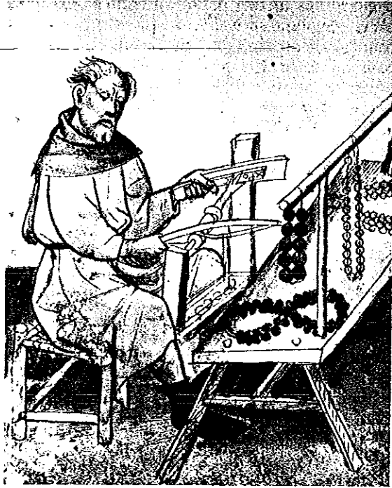
Figure 35: Rosary bead maker using a bow-driven lathe or drill, from the fifteenth-century Hausbuch der Mendelschen Zwölfbrüderstiftung (f. 13 v ) (For an account of the complete manuscript see Treue et al. 1965)
